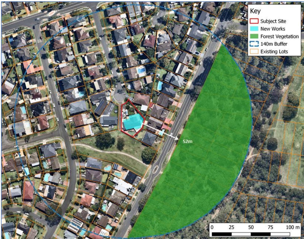
Figure 5. Hazardous vegetation affecting the subject building. Source: NearMap (2022) with overlays by BFCS P/L.
